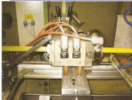
When the process stabilizes (after about five minutes) coextrusion of surface skin begins. Photo shows pultruded rod exiting the pultrusion die (left) and passing through co-extrusion system (center), where a yellow surface/cap layer is applied (right).
