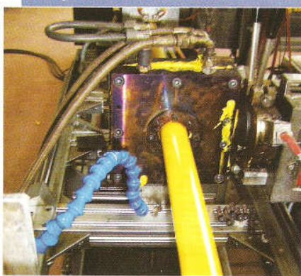
Pultruded rod with surface skin (cap layer) is pulled out of the coextrusion die. The blue, segmented hose sprays cool water on the rod as it exits the die to reduce cooldown time.
