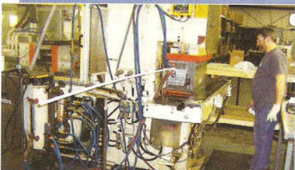
An 8-ft/2.4m section core rod is placed in the injection die. Long-fiber TPU is ram-injected into the die, forming threads on that section. After cooling, the rod is indexed downstream and threads are formed on the next and successive sections.
