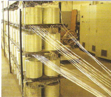
Glass roving is loaded onto racks, threaded through tensioners, and then drawn through the forming tooling, dies and pullers.
