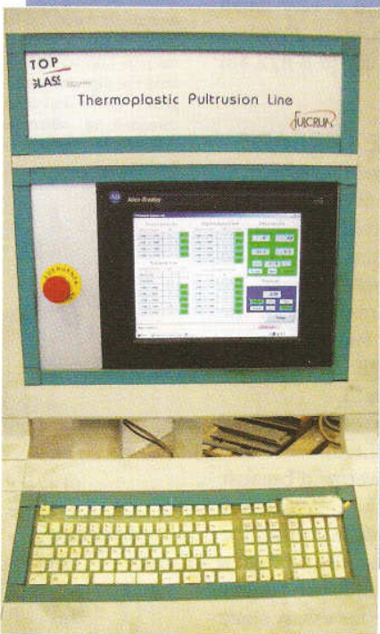
Resin and pultrusion/coextrusion dies are preheated to melt temperature, set and then monitored by Fulcrum's computerized control system (above). After resin feed is started, pultrusion process parameters are adjusted to achieve through wetout.
